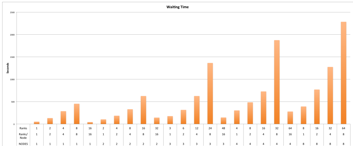
Figure A.12: Waiting time (s) per MPI rank/node for all to all neighbour data exchange over 1000 time steps (25 mil triangles, 10k non-spherical particles).
